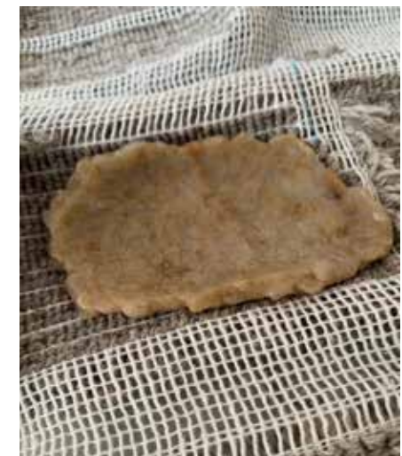
Figure 45: Application of Bacterial cellulose as Scaffold on hand-tufting prototype.
