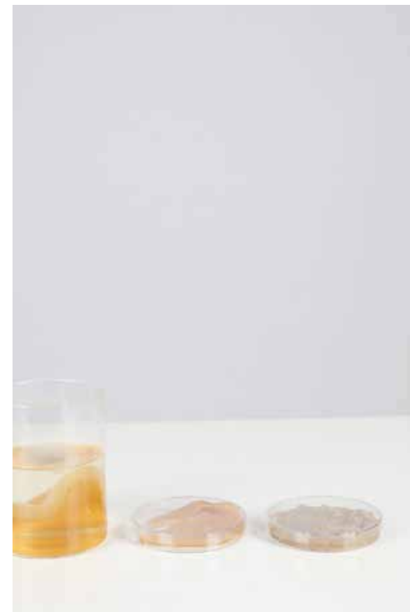
Figure 7: Bacterial cellulose, from scoby to pulp.
