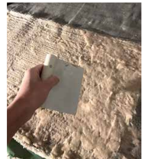
Figure 46: Application of Bacterial cellulose as Scaffold on hand-tufting prototype.
