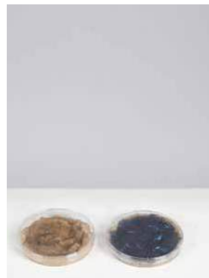
Figure 10: Bacterial cellulose pulp tests with mica mineral.- By the author
