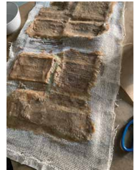
Figure 44: Application of Bacterial cellulose as Scaffold on hand-tufting prototype.
