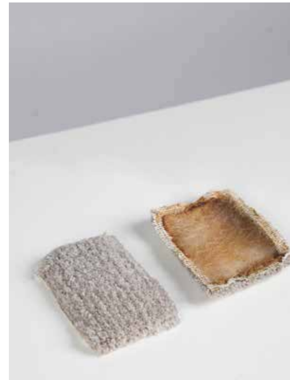
Figure 43: Bacterial cellulose as Scaffold on hand-tufting sample.
